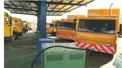
Sevilla is one of the first cities in the world using vehicles with electric propulsion for the collection of urban waste. The use of bimodal waste collecting vehicles (compactors) in the historic centre of Sevilla provides important advantages over conventional collection vehicles. The practical benefits of this technology also include lower emissions and environmental noise at low speeds compared to conventional vehicles.
